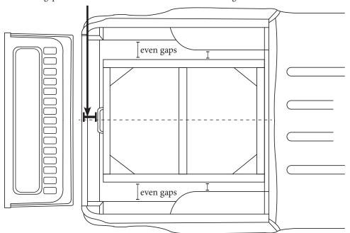
**2** Centre the frame in the middle of the tub allowing even gaps between wheel arches.
