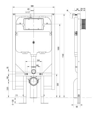
The concealed, dual flush cistern with frame is made from high density polyethylene, incorporating inbuilt overflow. This cistern is suitable for in-wall and under counter installation.
