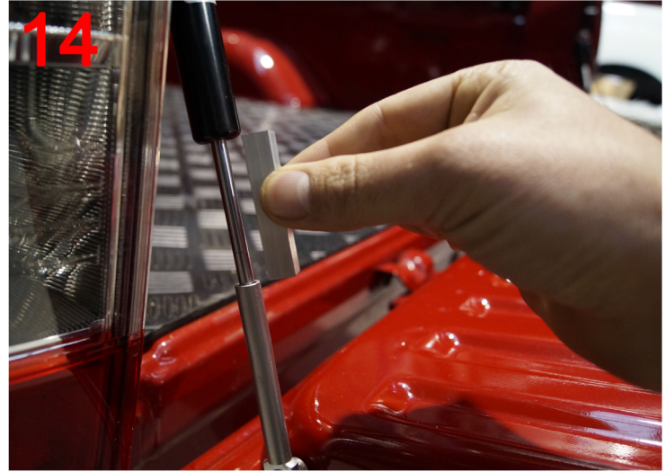
14: Repeat the process on the passenger side for the EASY UP strut removing the spacer once installed
