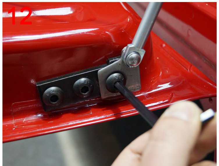
12: Place the bottom of the strut over the tailgate bracket and screw in the 3rd bolt
