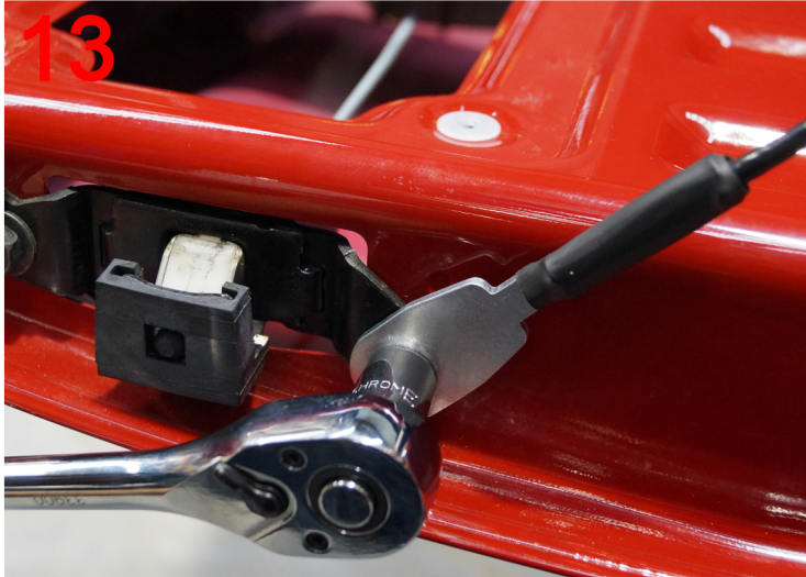
13: Reinstall the cable bolt removed in step 2 placing the cable on first
