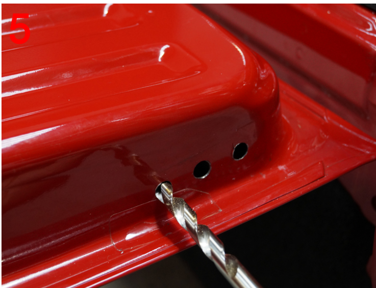
5: Drill the three holes to 10mm TIP: drill smaller holes first to help locate the bit
