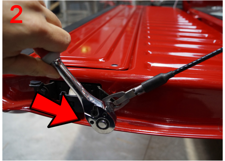
2: Remove strap bolt from the tailgate
