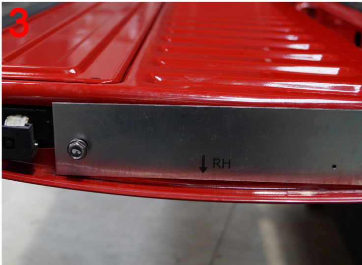
3: Bolt on the drilling template as pictured
