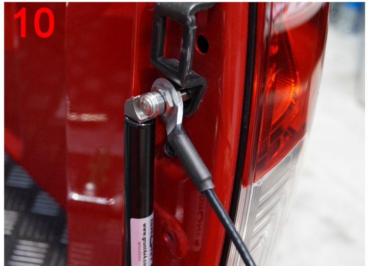
10: Install the strut and new cable supplied as shown
