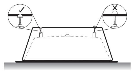
**STEP 2** Return the bath to its feet to check that the bath sits level and adjust legs to compensate for any variations in floor level if required.
