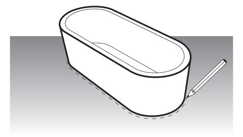
**STEP 5** Using the appropriate silicone for the surface type, apply silicone inside the bath outline. Line the bath up with the outline and place the bath in position. Allow at least 24 hours for the silicone to set before using the bath.
