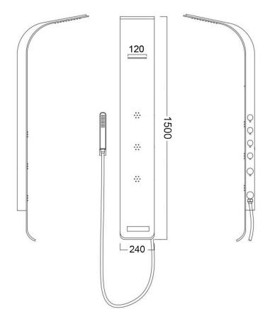
The Synergii shower panel is created from aluminum alloy with durable stainless steel hoses and brass bodies for the body jets.
