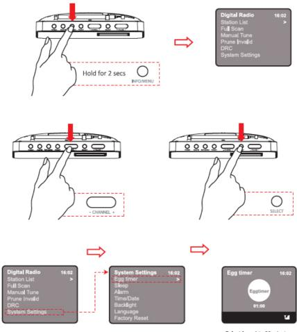
Select from 1 to 99 minutes; press POWER to stop the buzzer,
