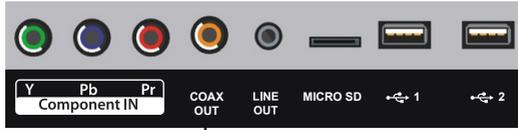
Use a coaxial cable (not included) to connect the unit with amplifier or other audio decoding device for coaxial audio signal output.
