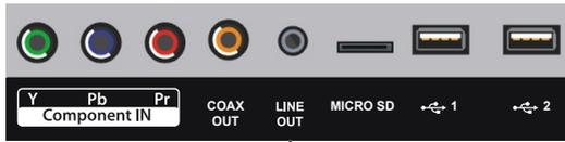
Line Out socket outputs audio at a low amplification level. Connect to an external digital audio device using a 3.5mm audio cable (cable is not included) and use the device to control the sound output.
