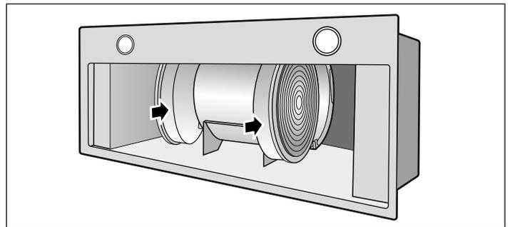
4. Install the metal grease filters.
