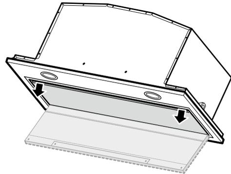
2. Open the lock and fold down the metal grease filter.
