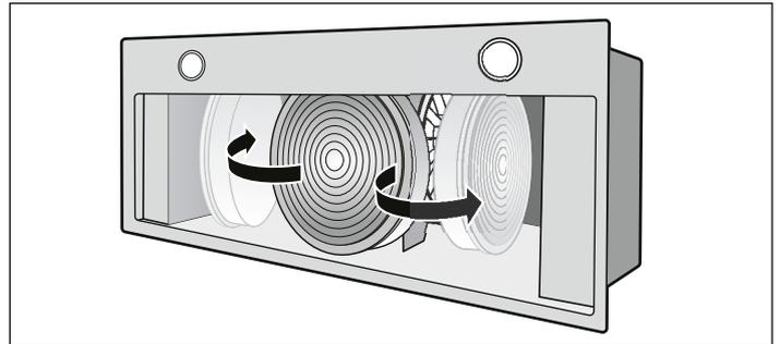
3. Carefully slide the new activated charcoal filter into the retainer.
