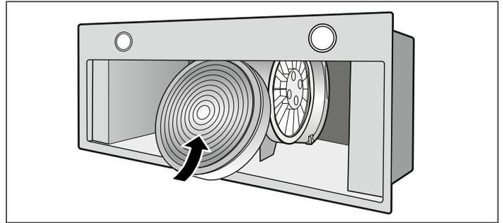
2. Guide the activated charcoal filter around the motor.
