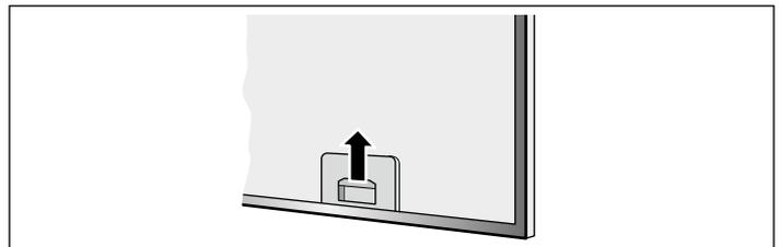
3. Take the metal grease filter out of the holder.
