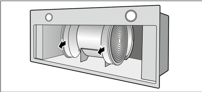
3. Guide the activated charcoal filter around the motor.
