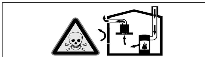
Room air-dependent heat-producing appliances (e.g. gas, oil, wood or coal-operated heaters, continuous flow heaters or water heaters) obtain combustion air from the room in which they are installed and discharge the exhaust gases into the open air through an exhaust gas system (e.g. a chimney).
