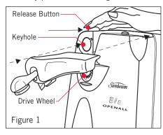
The Cutting Assembly fits into the keyhole opening at the top of the Open All™ can opener, above the Drive Wheel. Slide the Release Button to the right as the Cutting Assembly is inserted, it will "click" into position, with the release button returning to its original position.
